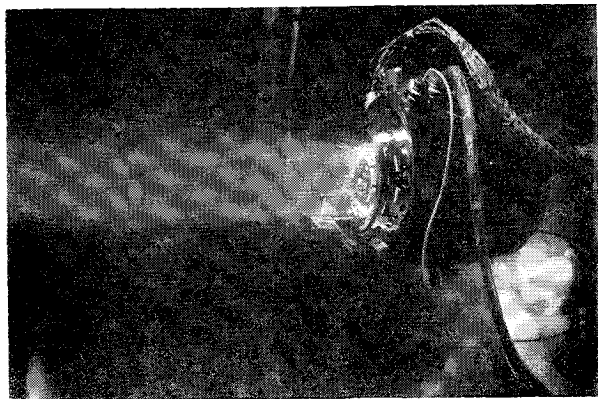
Fig. 6 Cesium ion beam emanating from an operating SERT I ion engine in a vacuum chamber
